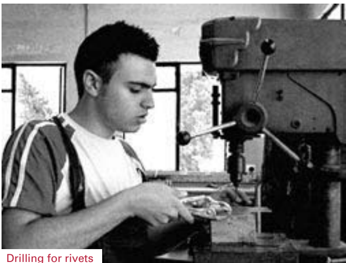
Drilling for rivets
