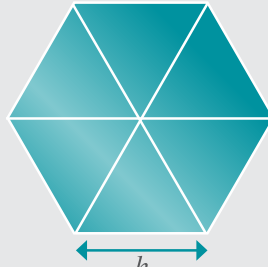
Figure 4: The area of a regular hexagon can be found by splitting it into 6 equilateral triangles.
